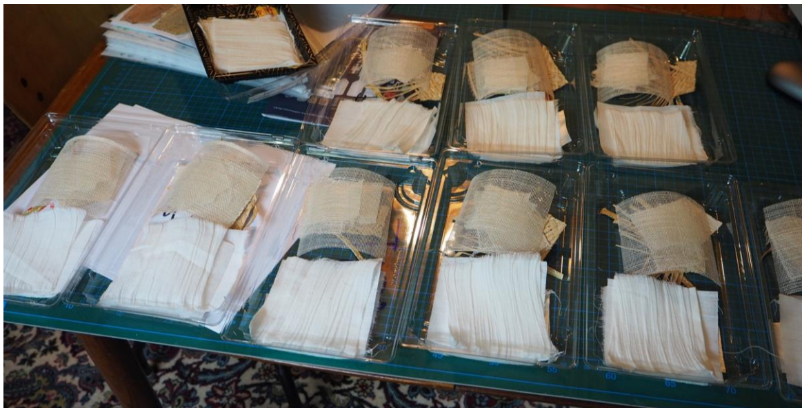
Preparation of swatches going into dyebaths. These are high and low processed plant fibres, and some regenerated fibres going into a cold-water fibre reactive dye bath.
