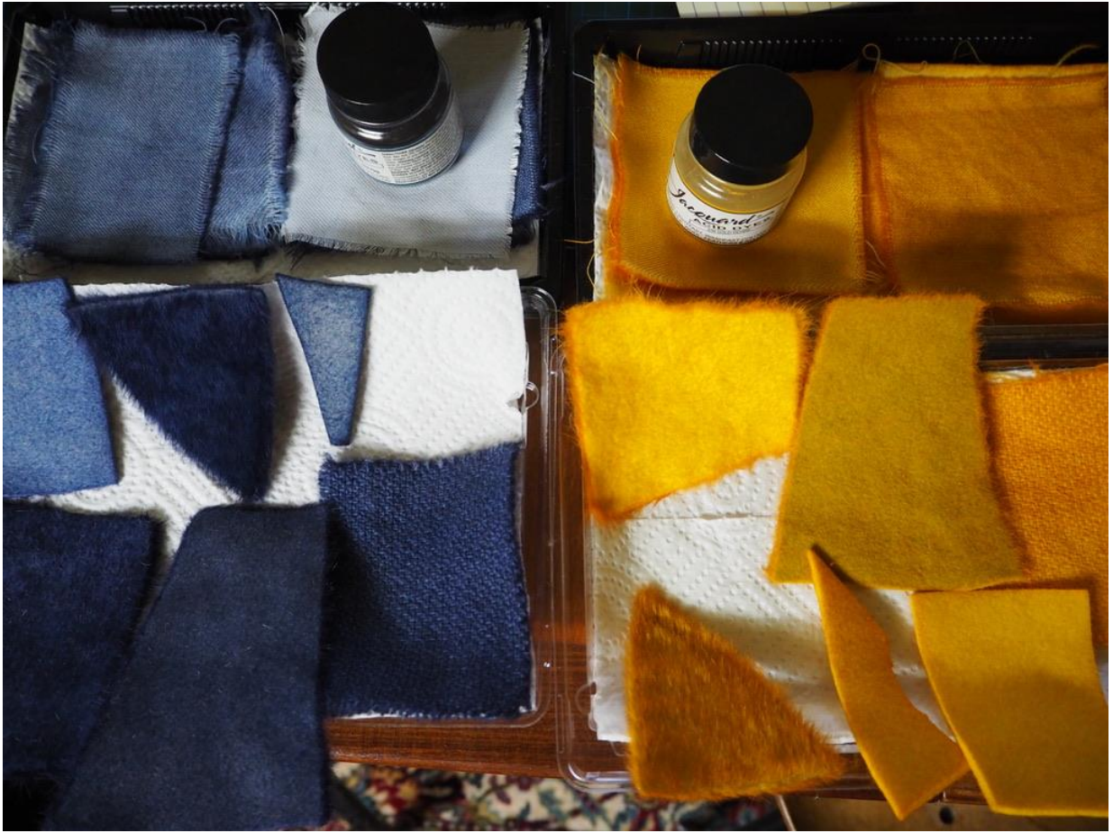
Wool fabric, wool and hair felt swatches after dyeing, rinsing and drying.
