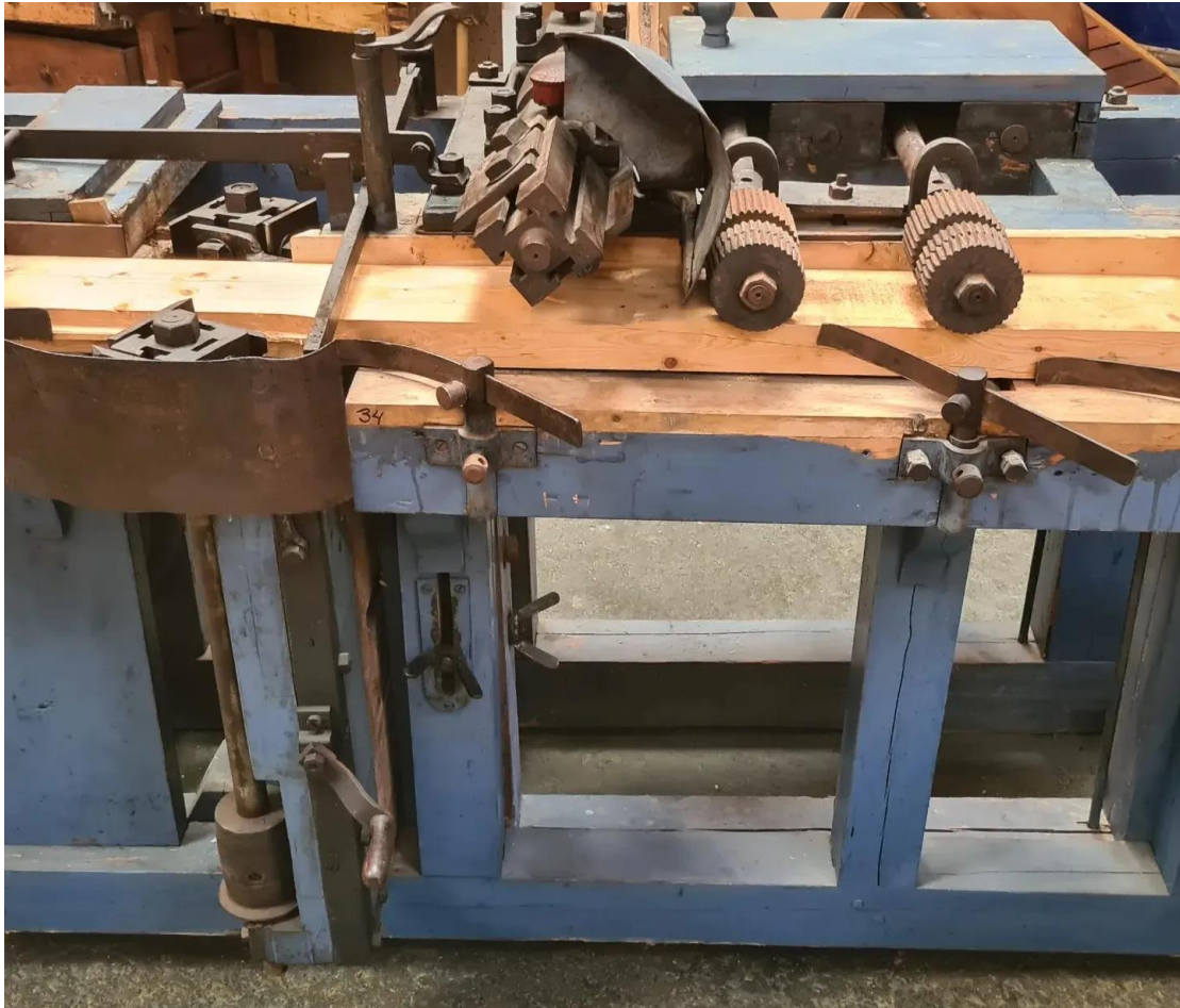
Trespindlet moulding i tre ca. 1920, Arvesund Jämtland.
